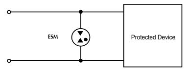
Signal circuits often run with no ground conductor. A ESM circuit located between the two signal lines offers differential mode protection by preventing the occurrence of large potential difference at the input of the equipment to be protected
